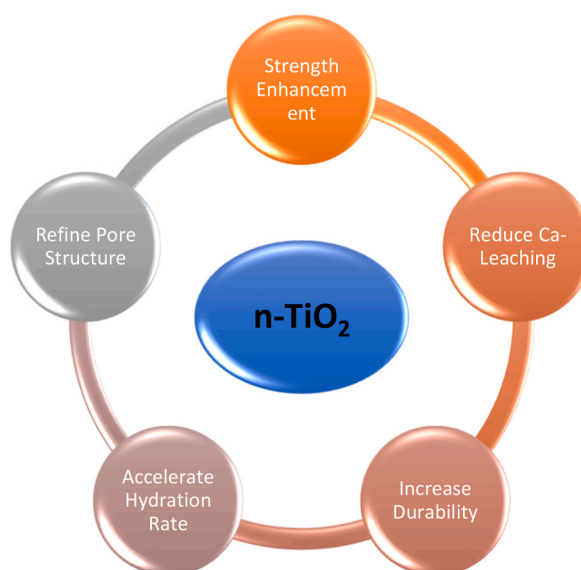
Fig. 4. Behavior of Nano- \text{TiO}_2 in the cement matrix and enhanced properties.
